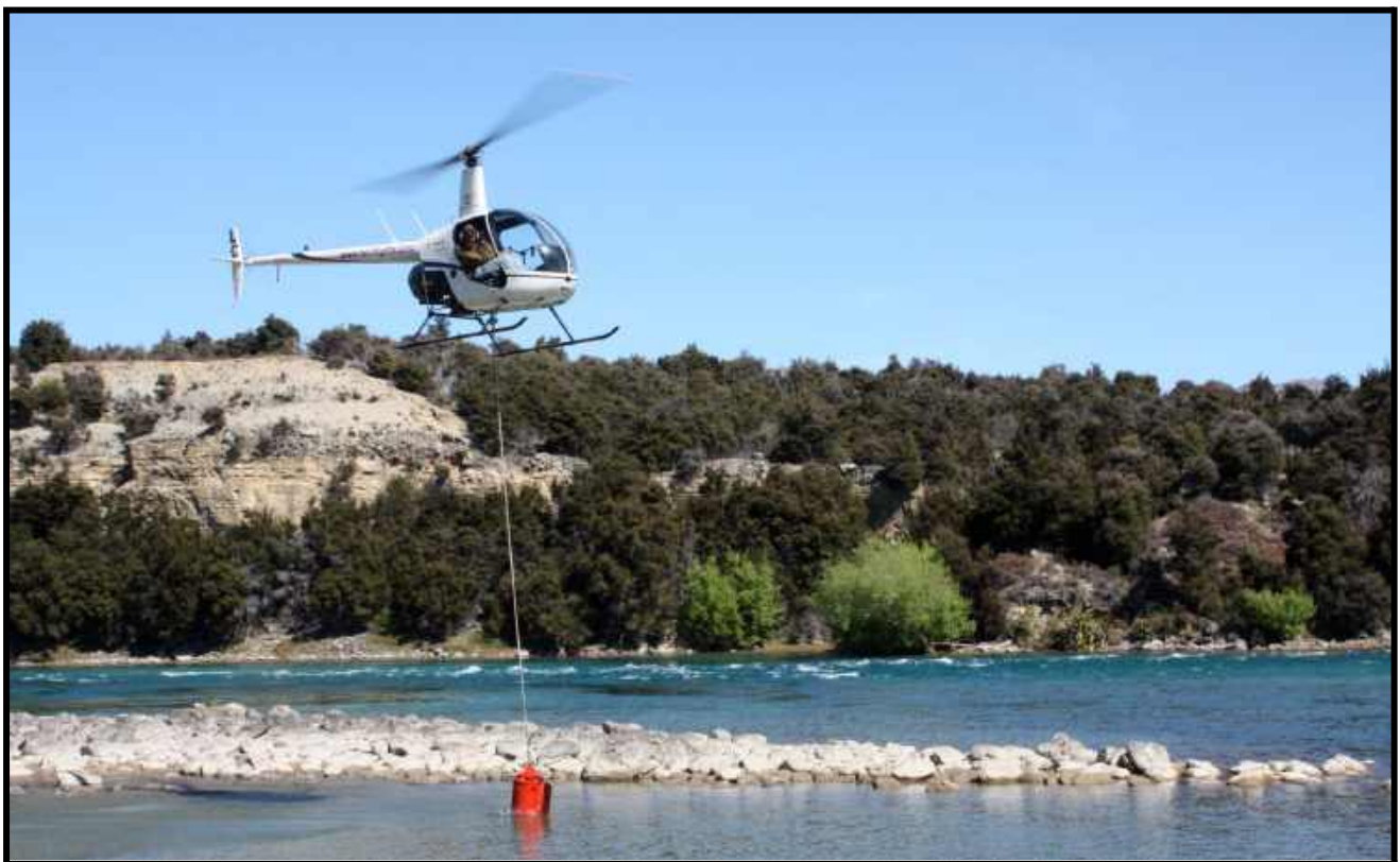
Figure 2. Student conducting a fire-bucket sling operation with a two-seat trainer (Robinson R22)
