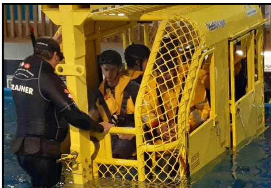
Figure 1. Students undertaking Helicopter Underwater Escape Training which improves their survivability in a real-world incident by 60%. This exercise (where they are forced underwater, flipped upside down) is overseen by an instructor, two safety divers, and you can notice emergency releases for all doors and seatbelts on the side of the training device.
